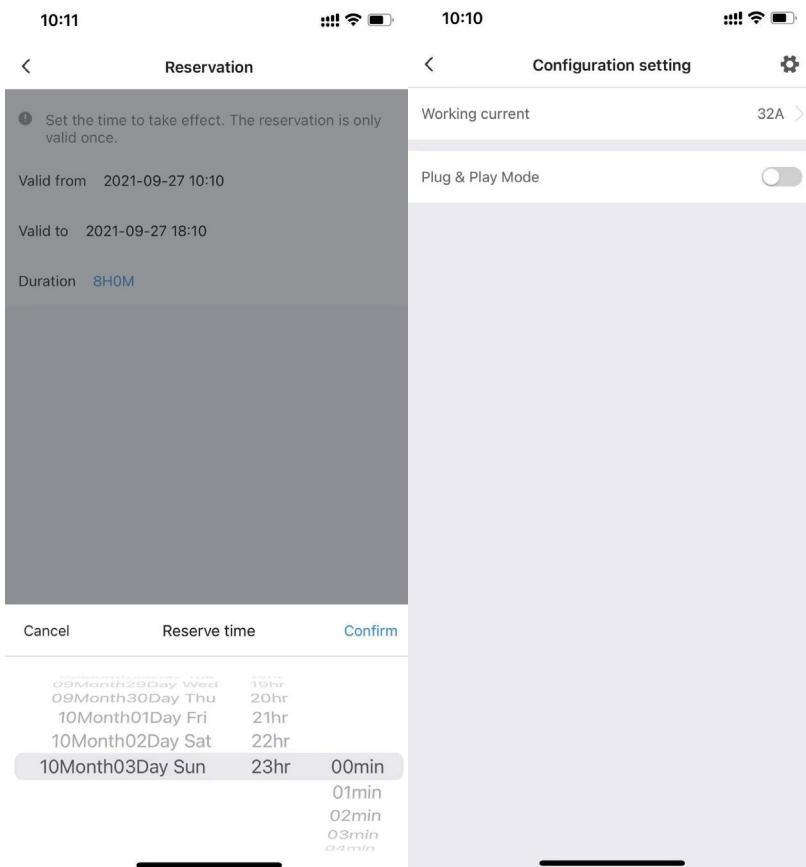
To set delay charging , charging end time by date , hour and minute , and to set the max charging current , and plug and play mode.
