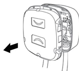
2. Remove the 7 screws around the internal panel and take the panel down.
