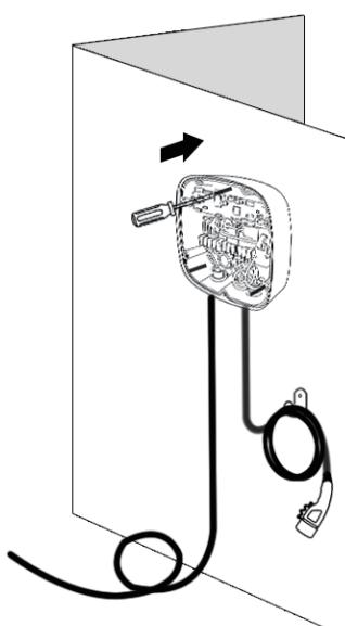
5. Mounting the disassembled back cover on the wall
