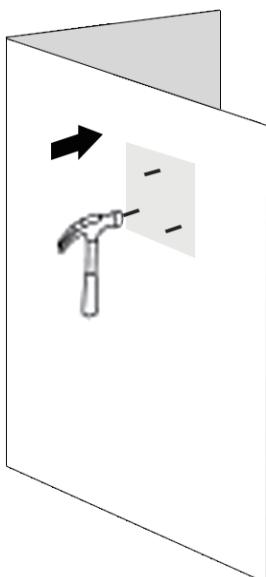
4. Tap the expansion bolts into the mounting holes.
