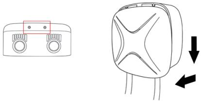
1. Remove the two screws at the bottom of the cover plate, then push down and remove it from the wallbox.
