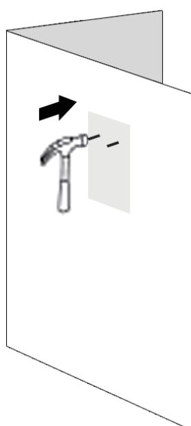
2. Tap the expansion bolts into the mounting holes.
