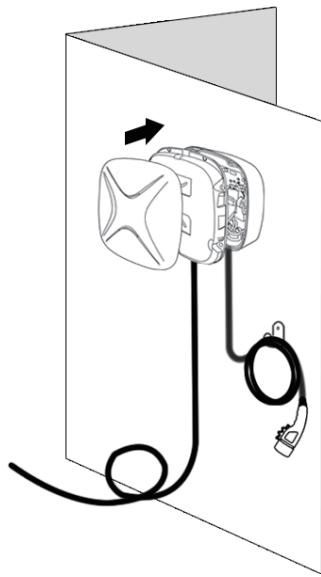
6. Install the removed front panel back in order.
