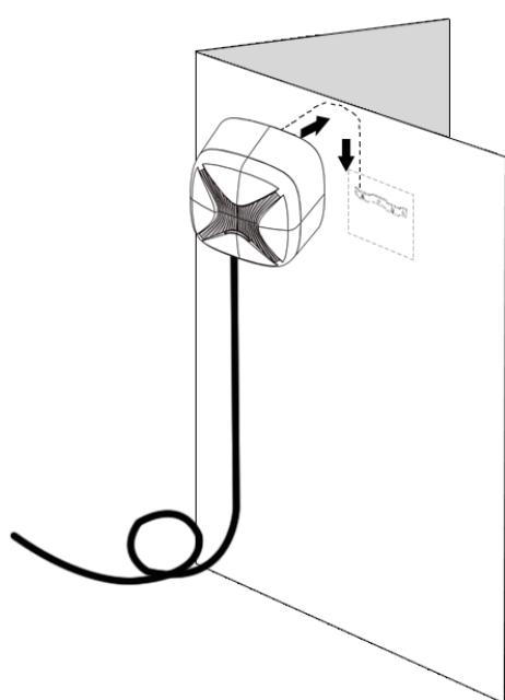
4. Place the wallbox in from the top down and fix it to the back plate
