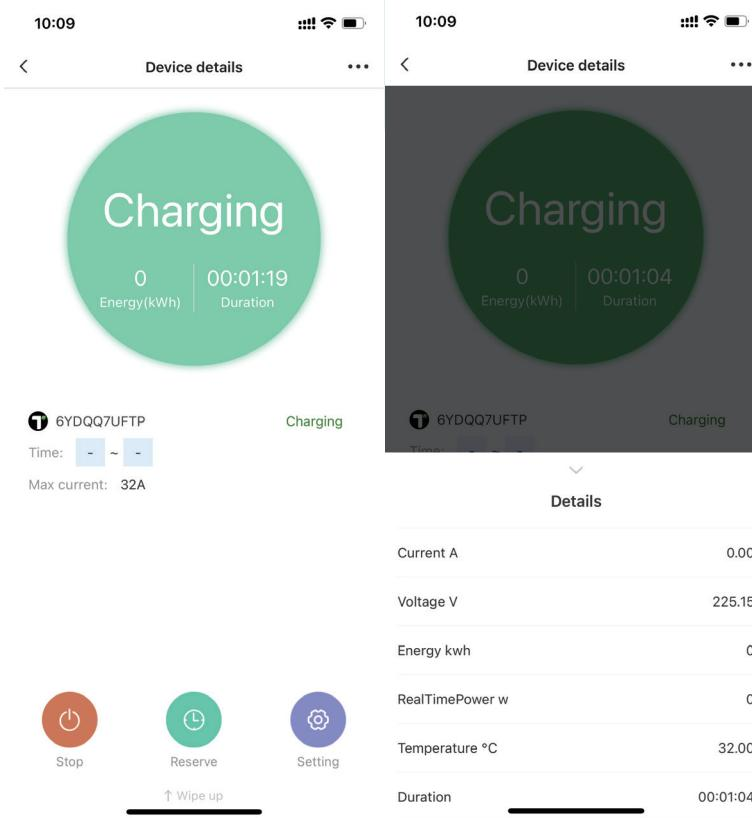
According to your need to enter charging mode, scheduling charging, current adjusted mode or set plug and play mode ,etc to control your ev charger
