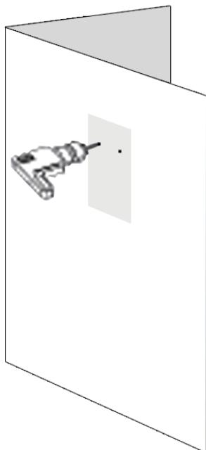
1. Use a drill to make mounting holes in suitable locations on the wall.
